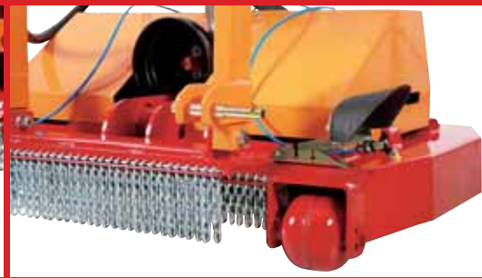
Herbicide spraying head adjustable in height and depth
